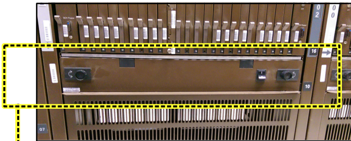
DMS-100 NTRX91AA FAN UNIT w/ EXISTING FANS
