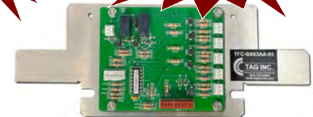
(1) # TFC-BX63AA-01 Fan Alarm Control Board w/ Mounting Bracket
