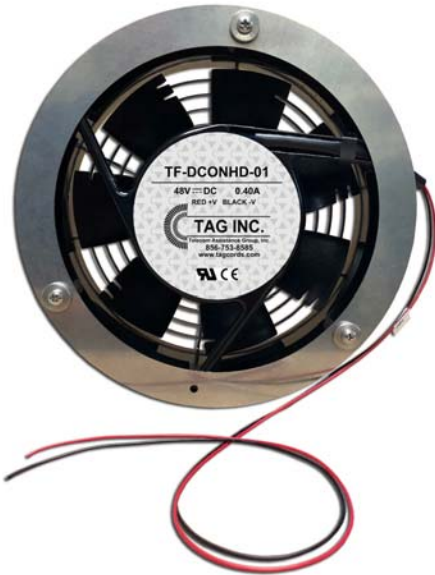
FTR UPN # TF-DCONHD-01 48 Volt Replacement Fan for DCO Non High Density CMF Bay w/ 2 Wire Open End (for splicing) (Black -48V, Red +48 Return) Includes: Guard Grill & (1) Butt Splice
