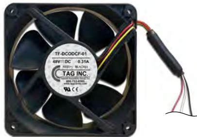
FTR UPN # TF-DCONHD-01 48 Volt Replacement Fan for DCO Non High Density CMF Bay w/ 2 Wire Open End (for splicing) (Black -48V, Red +48 Return) Includes: Guard Grill & (1) Butt Splice
