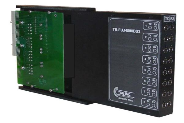
The TB-FUJ4500DS3 provides a quick method to transmit an acceptable test signal from the FLASHWAVE 4500 DS3 card slots to the DSX-3. At the DSX-3, Tester 2 will loop the signal back to the TB-FUJ4500DS3 and determine if the signal is acceptable for system turnup. The wiring label indicates Transmit (Tx) and Receive (Rx) 440A jacks for the 8 DS3 circuits. The TB-FUJ4500DS3 is used on non-powered systems.
