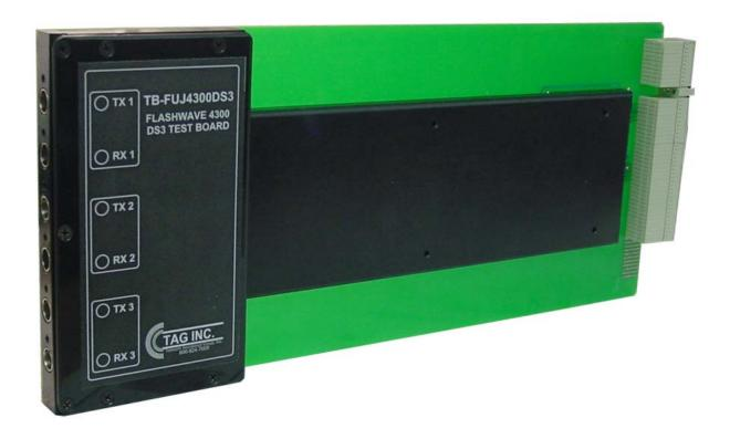
The TB-FUJ4300DS3 provides a quick method to transmit an acceptable test signal from the FLASHWAVE 4300 DS3 card slots to the DSX-3. At the DSX-3, Tester 2 will loop the signal back to the TB-FUJ4300DS3 and determine if the signal is acceptable for system turnup. The wiring label indicates Transmit (Tx) and Receive (Rx) 440A jacks for the 3 DS3 circuits. The TB-FUJ4500DS3 is used on non-powered systems.
