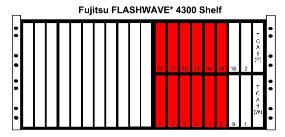
\*The (TB-FUJ4300DS3) FLASHWAVE 4300 DS3 Test Board will plug into slots (3-8) & (10-15) color coded red.
