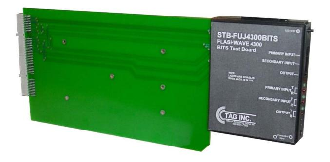
The STB-FUJ4300BITS provides a quick method to verify continuity, as well as, transmit a test signal from the FLASHWAVE 4300 BITS card slots to the DSX-1. At the DSX-1, Tester 2 will use a continuity test probe to verify that the BITS card slot is properly wired. Tester 2 is also capable of looping a test signal back to the STB-FUJ4300BITS and Tester 1 can determine if the signal is acceptable for system turn up. The STB-FUJ4300BITS is used on non-powered systems.
