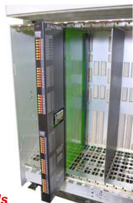
1. Press LED test button. If ALL LED's do not illuminate, replace battery.
