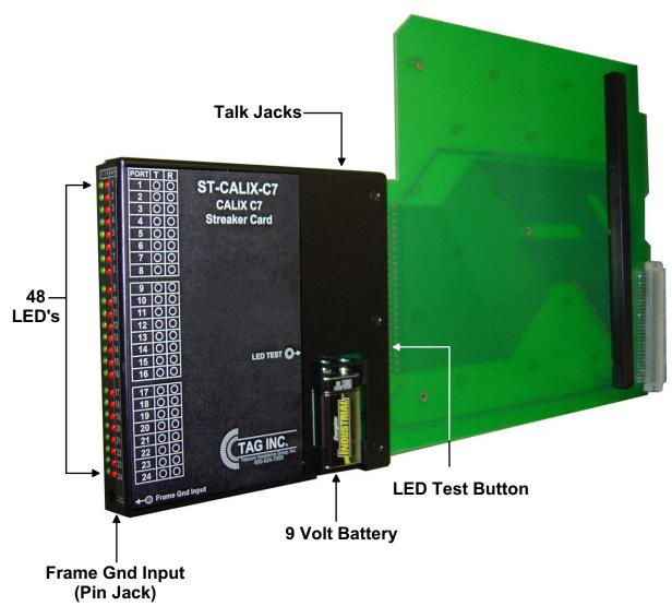
The ST-CALIX-C7 provides a quick method to "streak"- verify wiring via LED's from the backplane of the Calix C7 to the Frame. At the Frame simply ground the corresponding pins and the ST-CALIX-C7 will light the LED associated with that connection.
