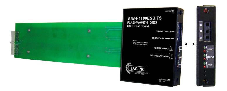
The STB-F4100ESBITS provides a quick method to verify continuity, as well as, transmit a test signal from the FLASHWAVE 4100ES BITS card slots to the DSX-1. At the DSX-1, Tester 2 will use a continuity test probe to verify that the BITS card slot is properly wired. Tester 2 is also capable of looping a test signal back to the STB-F4100ESBITS and Tester 1 can determine if the signal is acceptable for system turn up. The STB-F4100ESBITS is used on non-powered systems.
