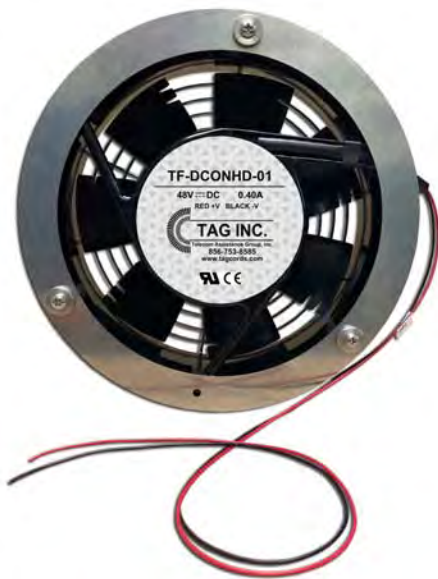
PN # TF-DCONHD-01 48 Volt Replacement Fan for DCO Non High Density CMF Bay w/ 2 Wire Open End (for splicing) (Black -48V, Red +48 Return) Includes: Guard Grill & (1) Butt Splice
