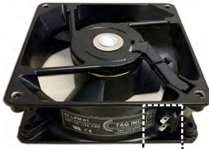
POWER PRONGS PLUG WIRES: YELLOW (+) BROWN (-)
