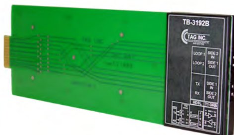
WINBUY # TB3192B 3190/3192 Office Repeater Test Board w/ Bantam Jacks
