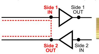
Plug Bantam to Bantam cord into Side 1 In and Side 2 Out
