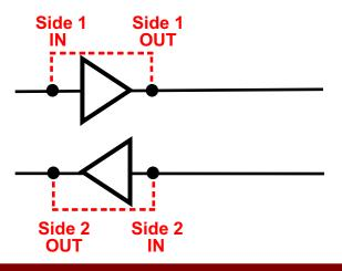
Plug Bantam to Bantam cord into Side 1 In and Side 1 Out & Side 2 In and Side 2 Out
