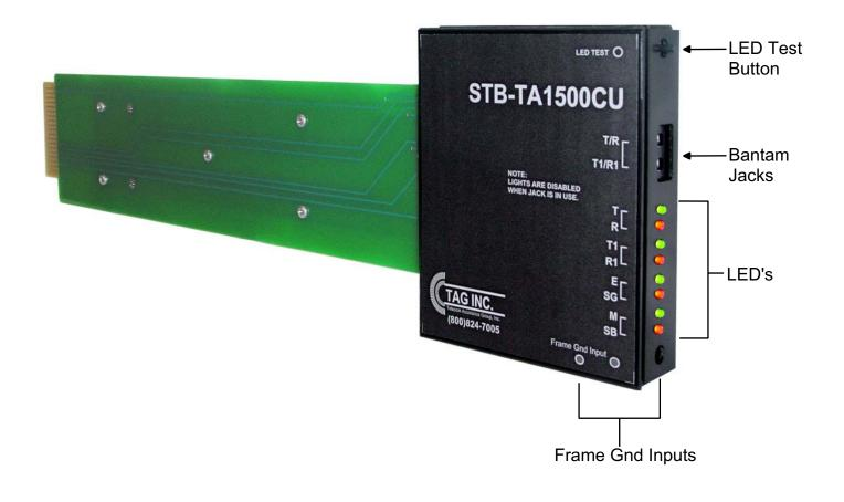
The STB-TA1500CU provides both continuity testing and jack access for signal acceptance testing from the Adtran Total Access 1500 Channel Unit card slot to the cross-connect wiring points. It has 8 LED's that correspond to the backplane wiring of the Channel Unit. The STB-TA1500CU has two (2) bantam jacks for metallic access to tip & ring pairs. It also has an LED test button, pin jacks for connection to the frame ground and a 9 volt battery to power the LED's.
