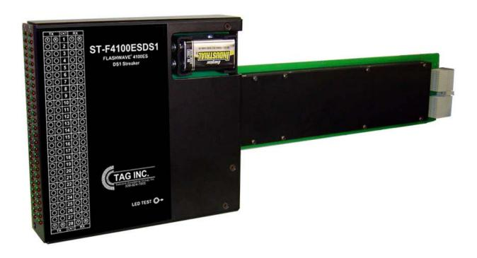
The ST-F4100ESDS1 provides a quick method to verify wiring continuity "streak" from the FLASHWAVE 4100ES DS1 card slots to the DSX-1. At the DSX-1, Tester 2 will ground the connection point and the ST-F4100ESDS1 will light the LED associated with that connection. The wiring label indicates LED's for 28 DS1 circuits. The ST-F4100ESDS1 is powered by a 9-Volt battery.
