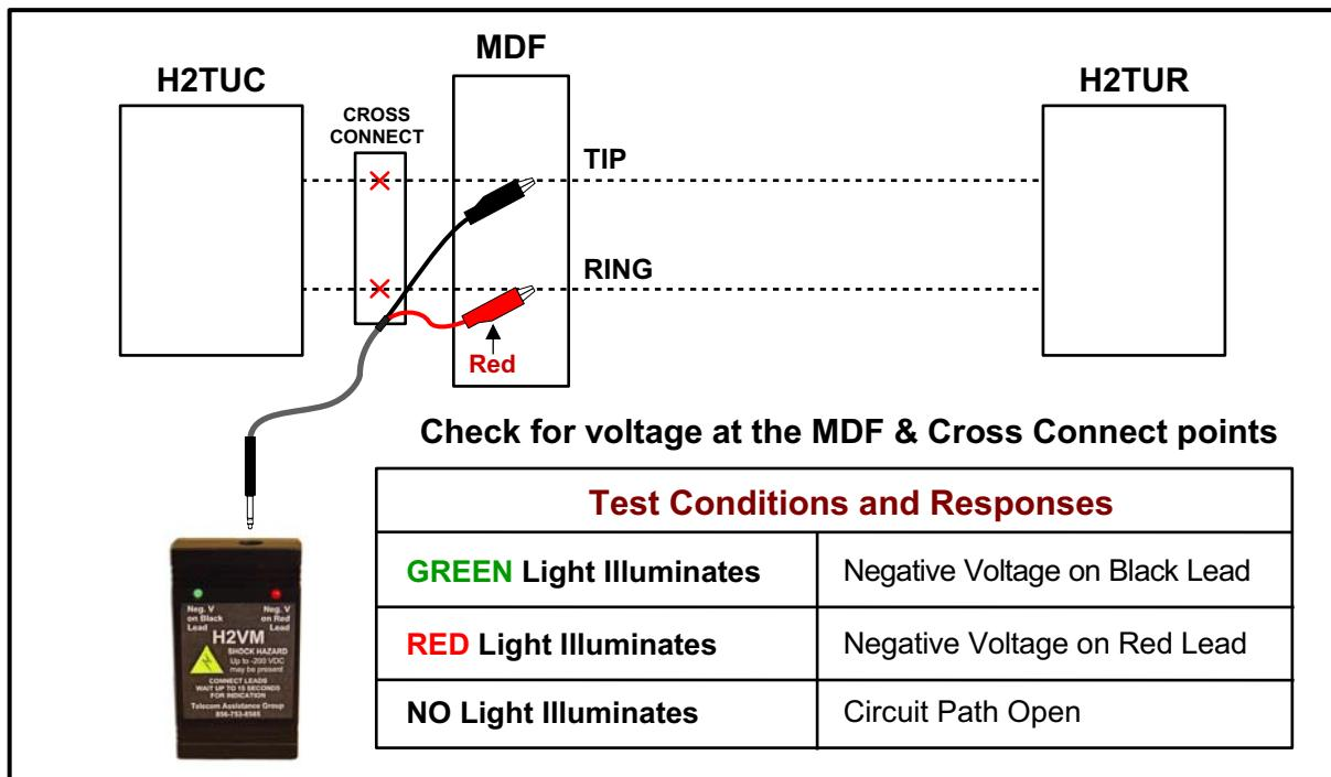
**4 Wire (Perform all tests with cable pairs open)**
