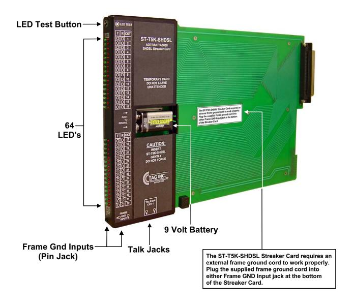
The ST-T5K-SHDSL provides a quick method to "streak", verify wiring via LED's, from the backplane of the Adtran TA5000 to the Frame. At the Frame simply ground the corresponding pins and the ST-T5K-SHDSL will light the LED associated with that connection.
