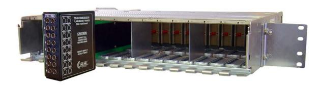
The (TB-F4100ESDS3-8) FLASHWAVE\* 4100ES DS3 Test Board will plug into slots configured for DS3
