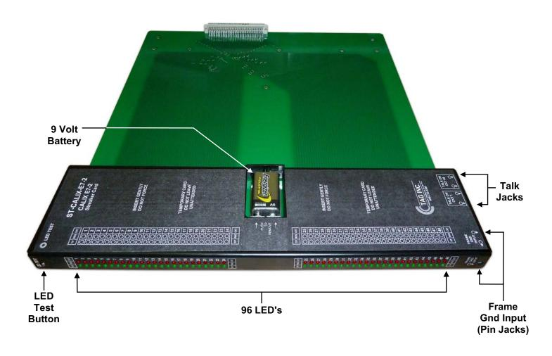
The ST-CALIX-E7-2 provides a quick method to "streak", verify wiring via LED's, from the backplane of the Calix E7-2 to the Frame. At the Frame simply ground the corresponding pins and the ST-CALIX-E7-2 will light the LED associated with that connection.
