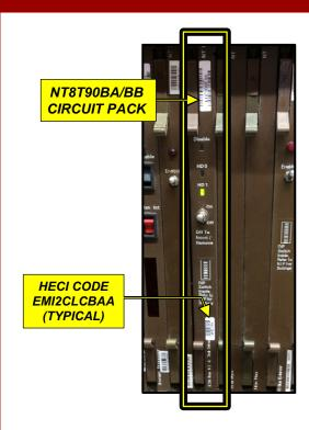
The procedure on the following pages details removing mechanical Hard Drives (HD) on DMS10 NT8T90BA/BB circuit packs & replacing them with a NEW TAG Solid State SCSI Drive (PN # TSD-8T90BB).
