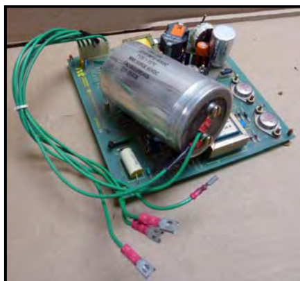
24VAC POWER SUPPLY UNIT DETACHED FROM THE DMS-100 NT3X90AA FAN UNIT
