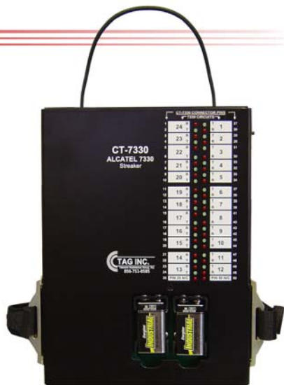
(1) CT-7330 Alcatel 7330 Streaker Unit w/ LED's
