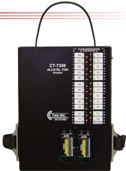
(1) CT-7330 Alcatel 7330 Streaker Unit w/ LED's
