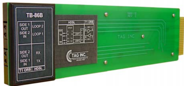
TB-86B "DDM Plus" Office Repeater Test Board w/ Bantam Jacks
