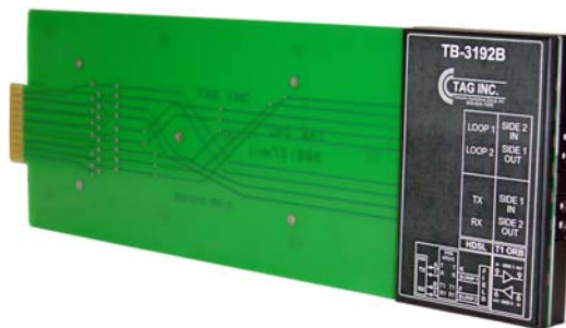
TB-3192B 3190/3192 Office Repeater Test Board w/ Bantam Jacks
