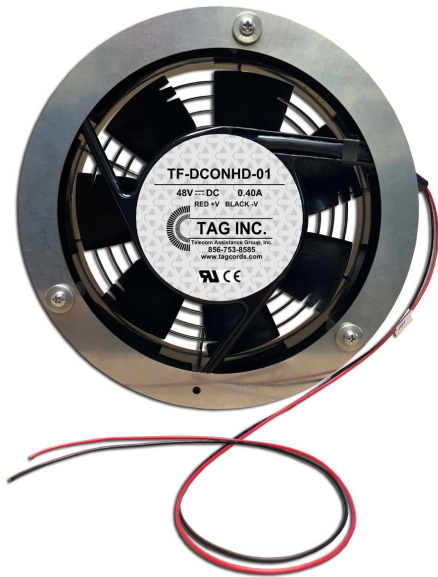
PN # TF-DCONHD-01 48 Volt Replacement Fan for DCO Non High Density CMF Bay w/ 2 Wire Open End (for splicing) (Black -48V, Red +48 Return) Includes: Guard Grill & (1) Butt Splice
