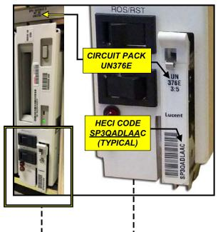
5ESS UN376 CIRCUIT PACK WITH AN <u>OLD</u> DAT DRIVE. THE TAG DAT DRIVE (# TSDT-5ESS-01) IS USED ON 5ESS UN376E & UN376F CIRCUIT PACKS.
