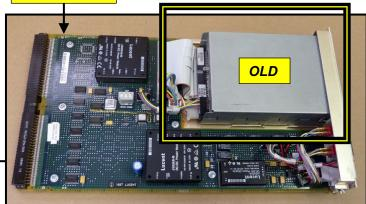
5ESS UN376 CIRCUIT PACK WITH THE OLD DEFECTIVE DRIVE REMOVED.
