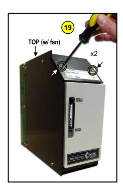
**19.** Use the TORX screwdriver to replace the (2) screws on the slanted top / front area of the module as shown.
