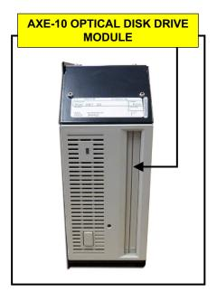
The procedure on the following pages details removing the failing Optical Disk Drive on an Ericsson AXE-10 Module & replacing it with a <u>NEW</u> TAG Solid State SCSI Tape Drive (# TSDT-AXE10-02).
