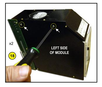
**18.** Use the TORX screwdriver to replace the (2) screws on the top of the left side of the module as shown.
