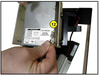
**12.** Attach the Ground faston connector to the # TSDT-AXE10-02 as shown.
