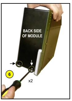
**6.** Use the TORX screwdriver to remove the (2) screws at the bottom of the back side of the module as shown. Set the screws aside for later use.
