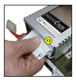
**14.** Attach the power cable to the #TSD-AXE10-02.
