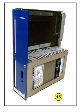
**15.** Install the AXE-10 Module with the NEW TAG Hard Drive back into the shelf according to Ericsson install & turn up procedures.
