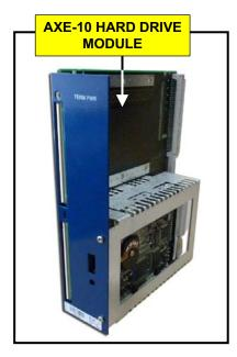
The procedure on the following pages details removing the failing Hard Drive on an Ericsson AXE-10 Module & replacing it with a <u>NEW</u> TAG Solid State SCSI Hard Drive (# TSD-AXE10-02).
