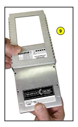
**11.** Place the metal drive carrier with the <a href="NEW">NEW</a> TAG Hard Drive into position on the AXE-10 Module.
