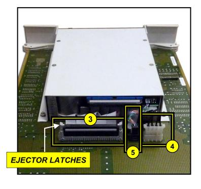
**6.** Remove the (4) screws attaching the metal mounting carrier on the circuit pack to the OLD tape drive.
