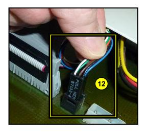
**13.** Connect the NEW power cable on the # TSDT-DCO-01 to the connector on the carrier.
