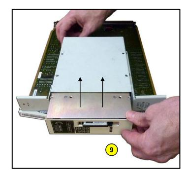
**10.** Position the # TSDT-DCO-01 almost flush with the cutout of the faceplate on the metal mounting carrier as shown below.
