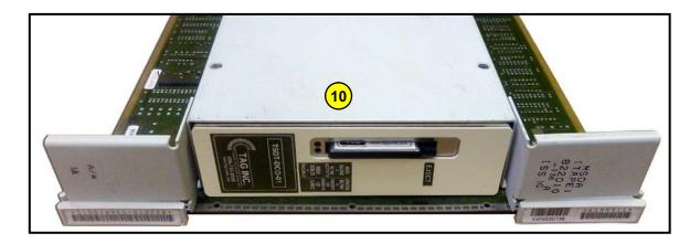
**11.** Connect the NEW ribbon cable on the # TSDT-DCO-01 to the connector on the carrier.
