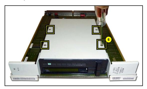
7. Carefully slide the OLD tape drive through the front area of the metal mounting carrier on the circuit pack.
