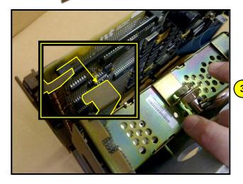
**3.** Separate the side panel from the main unit of the circuit pack by disconnecting the tabs from the notches as shown.
