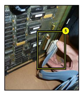
**5.** Remove the ribbon connector attaching the side panel to the main panel on the circuit pack. (Connector is seated tightly, pull hard to remove)
