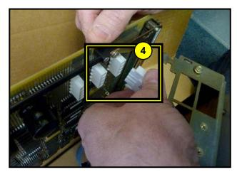
**4.** Remove the (2) connectors (P3 & P4) attaching the side panel to the main panel on the circuit pack. (Squeeze the tabs on the side of each connector)
