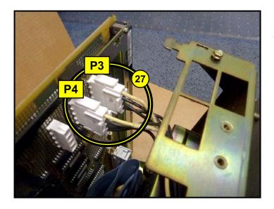
27. Plug the (2) connectors (P3 & P4) back into the side panel of the circuit pack as shown.
