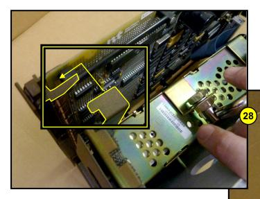
**28.** Reconnect tabs into notches of the side panel as shown.
