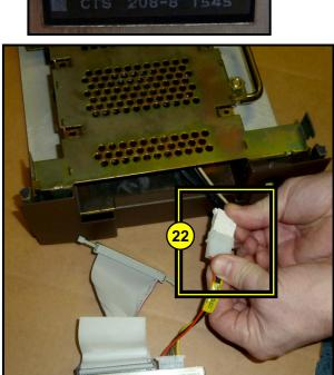
24. Attach the blue SCSI ribbon cable to the twisted extension SCSI ribbon cable on the # TSDT-9X44AD-02.
