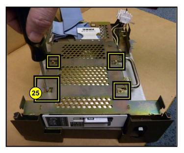
25. Secure the # TSDT-9X44AD-02 to the mounting cartridge on the circuit pack. Use a 1/8" hex nut driver to attach the (4) screws.
