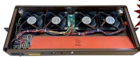
REFURBISHED DMS OPM, NT8X06AB FAN TRAY \* WITH (4) NEW 48V FANS & NEW ALARM CONTROL BOARD
