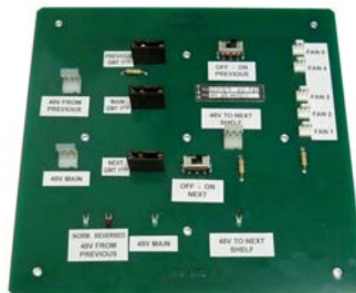
(1) Fan Control Board w/ Cabling & Mounting Hardware
