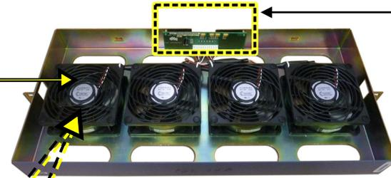
Kit is shown installed in existing DFA fan tray,
