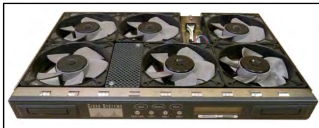
CISCO ONS 15454 FAN UNIT (6 FANS) (fan tray unit is not included)
