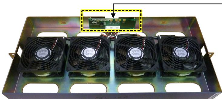
**KIT SHOWN INSTALLED IN EXISTING DFA FAN TRAY \***
