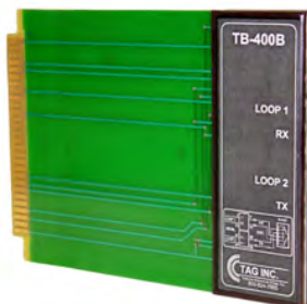
# TB400B HDSL Remote HRU-200/400 Mechanics w/ Bantam Jacks
