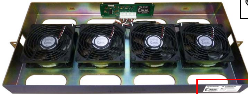
COMPLETED REFURB WITH ALL NEW FANS, NEW ALARM CONTROL BOARD & WARRANTY LABEL
